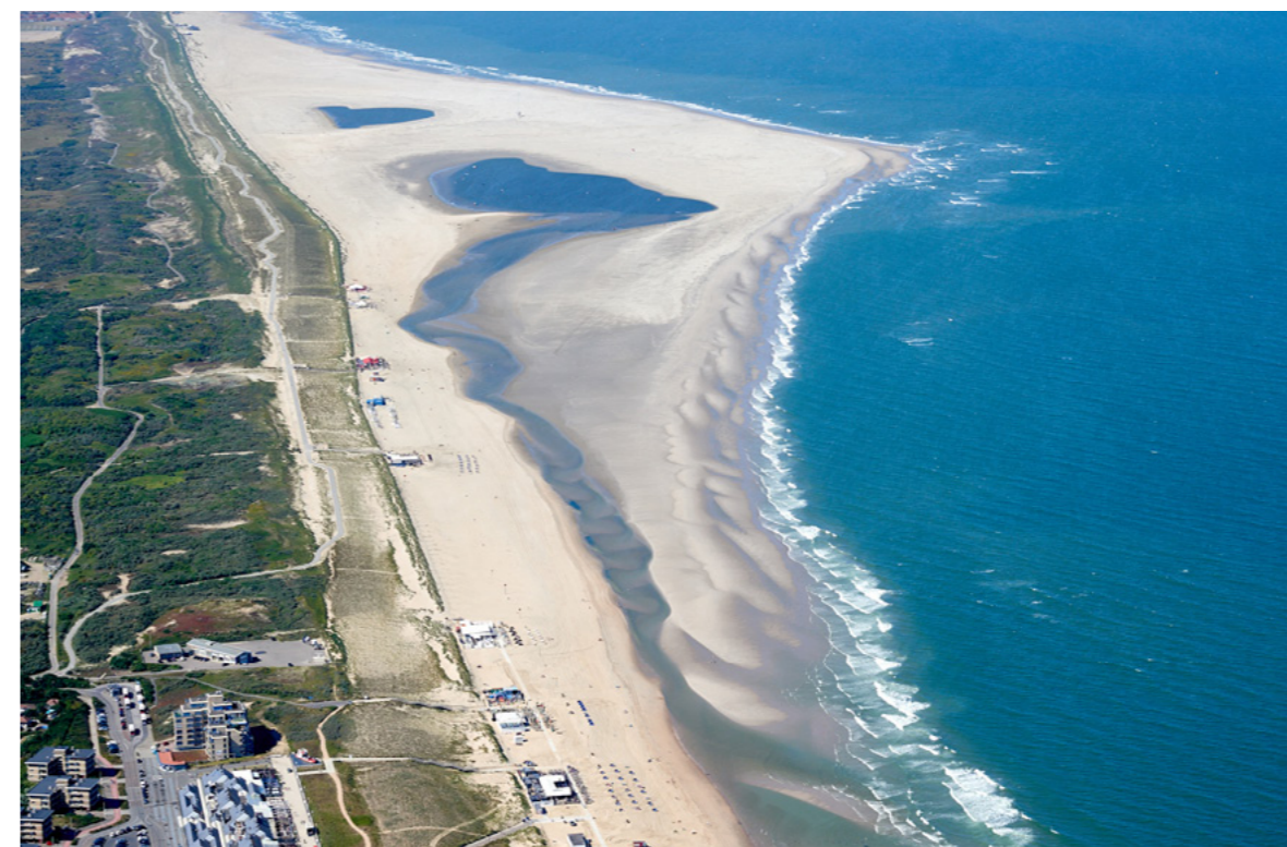
Sand suppletion off the Dutch coast (Building with Nature)
